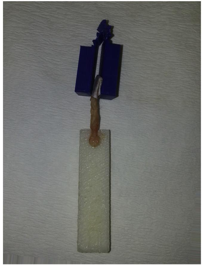
Fig. 4. The Achilles tendon and the mount used for mechanical testing.
